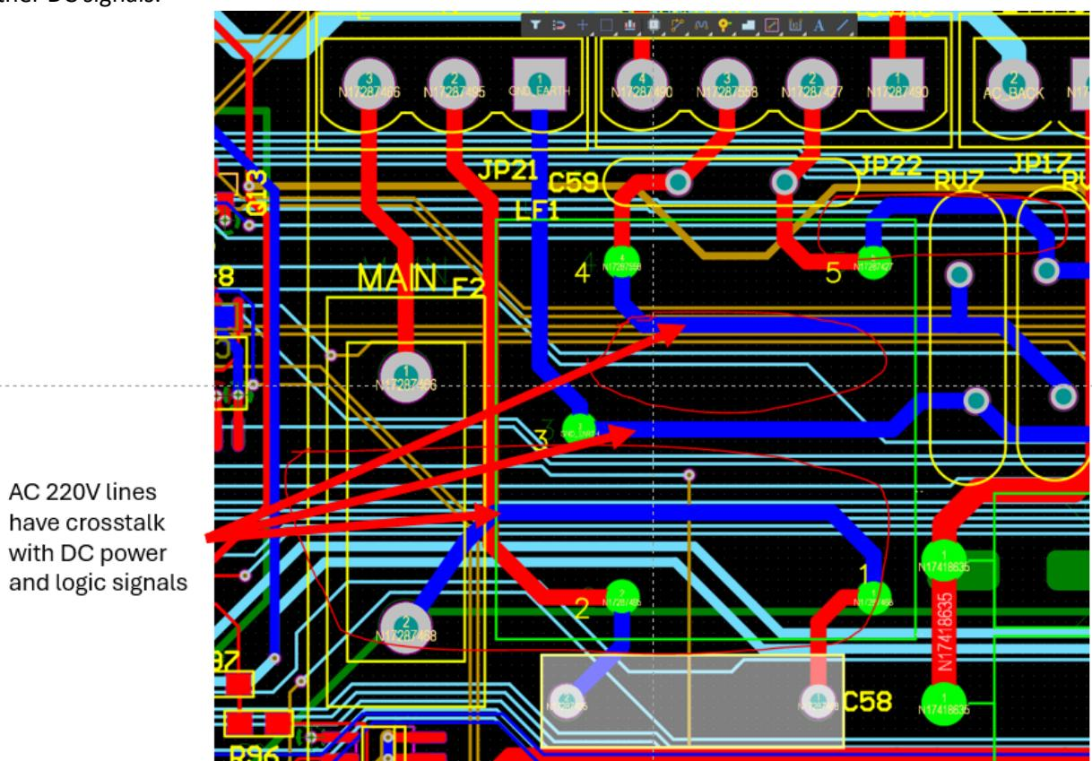
4) ESD/EMI Event propagation on PCBA via 24VAC line and impact of RV1 use case.
