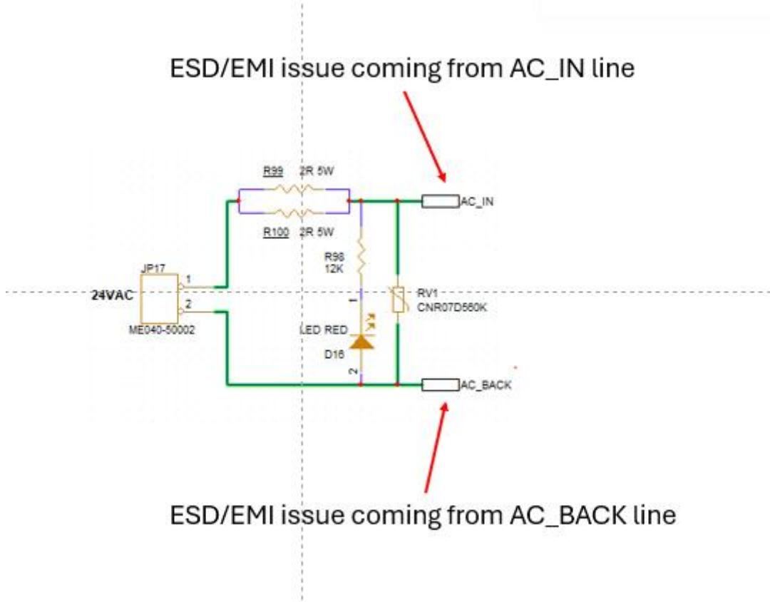
Action when both wires have the same voltage level: If both wires (AC\_IN and AC\_BACK) have the same overvoltage level at the same time, the varistor may not operate because the potential difference between the two wires will not be enough to activate it.
