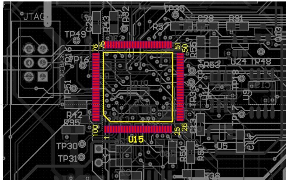
8) MCU, Wi-Fi and other logic circuits power inputs should be filtered with ferrite beads like in the picture. It will reduce or eliminate EMI event and save the power input of components.
