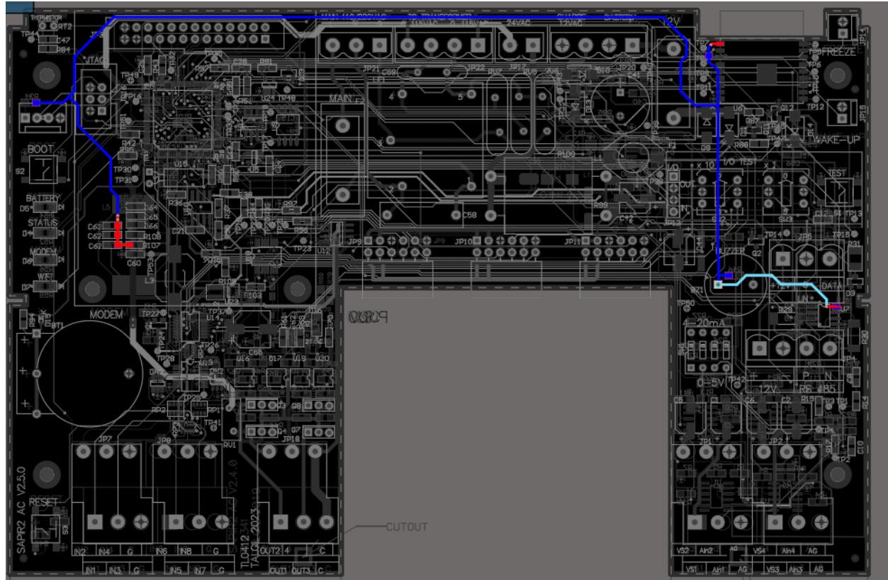
6) GND Field Signal should be polygon and not strip line.
